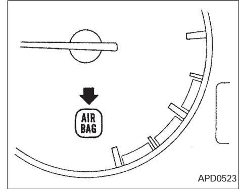
The supplemental air bag warning light, displaying <sup>AIR</sup>BAG in the instrument panel, monitors the circuits of the supplemental air bag system. The circuits monitored by the supplemental air bag warning light are the diagnosis sensor unit, supplemental air bag modules and all related wiring.
