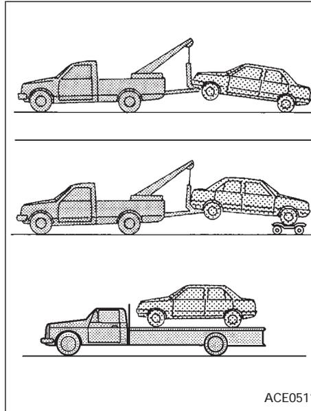
NISSAN recommends that your vehicle be towed with the driving (front) wheels off the ground as illustrated.
