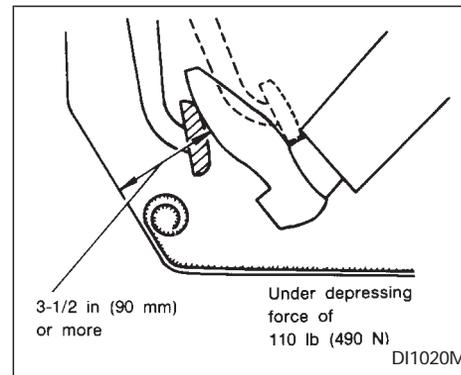
With the engine running, check the distance between the upper surface of the pedal and the metal floor. If it is out of the range shown above, see an authorized NISSAN dealer.
