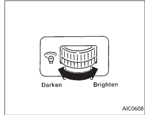
The instrument brightness control operates when the light switch is in the  $\text{DCE}$  or  $\text{DCE}$  position.
