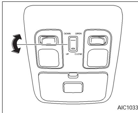
The sunroof operates only when the ignition key is in the ON position.
