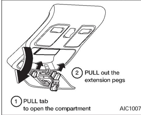
If the vehicle is equipped with a sunroof, there is an additional storage compartment in the map light unit. This storage compartment has been specially designed to hold some garage door transmitters. Some transmitters may not fit. When properly installed, the garage door transmitter can be activated while it is within the storage compartment.
