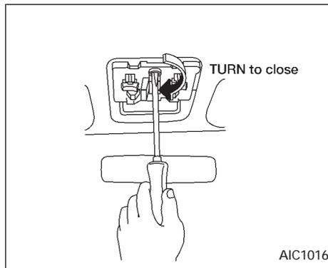
3. Using a wide blade screwdriver, turn the shaft clockwise to close the sunroof.
