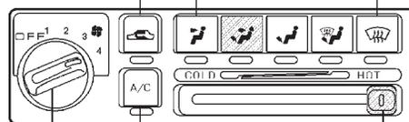
Fan control dial      Temperature control lever
