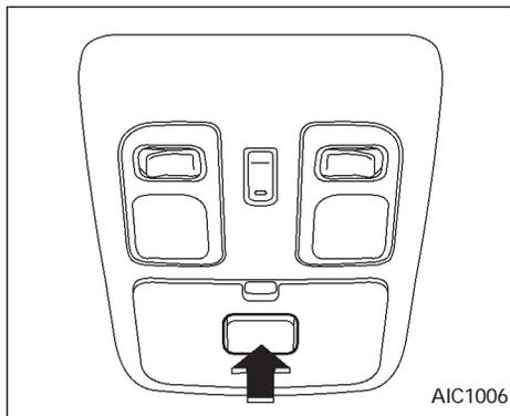
Once the garage door transmitter is installed, close the storage compartment door. Press the button on the center of the storage compartment door to operate the garage door transmitter.
