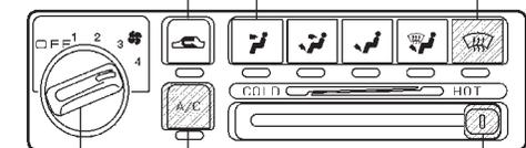
Fan control dial      Temperature control lever
