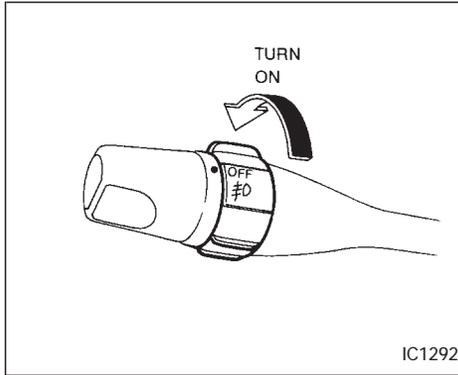
To turn the front fog lights on, rotate the switch to the
