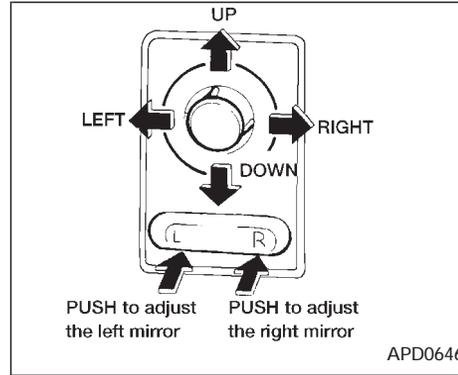
The outside mirror remote control only operates when the ignition switch is in the ACC or ON position.
