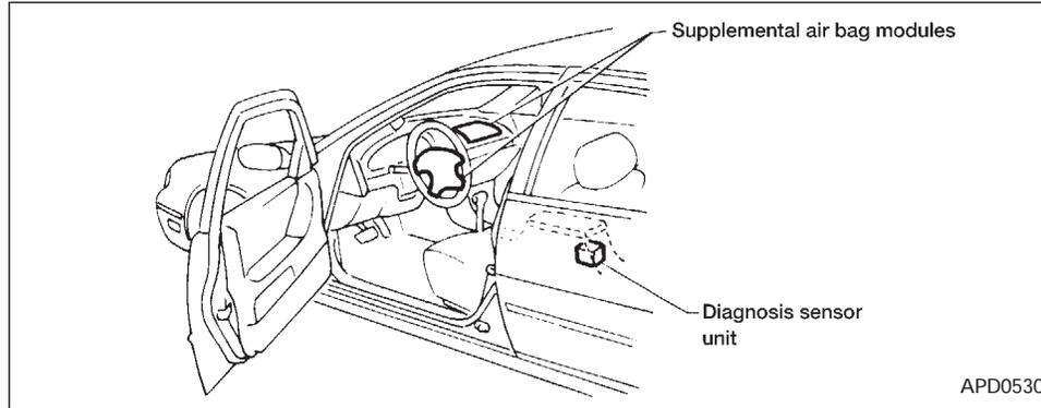
The driver supplemental air bag is located in the center of the steering wheel. The front passenger supplemental air bag is mounted in the dashboard above the glove box.
