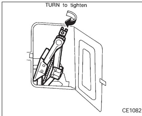
7. Install the jack in its storage area and tighten the jack screw clockwise.
