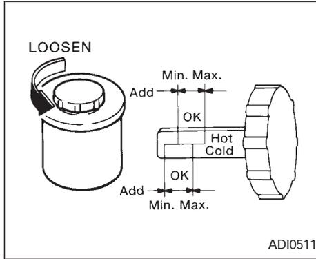
Check the fluid level in the reservoir. The fluid level should be checked using the HOT range on the dipstick at fluid temperatures of 122° to 176°F (50° to 80°C) or using the COLD range on the dipstick at fluid temperatures of 32° to 86°F (0° to 30°C).
