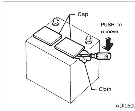
1. To remove the cap, gently pry between the battery cap and cover as illustrated. Use a cloth to protect the battery case.
