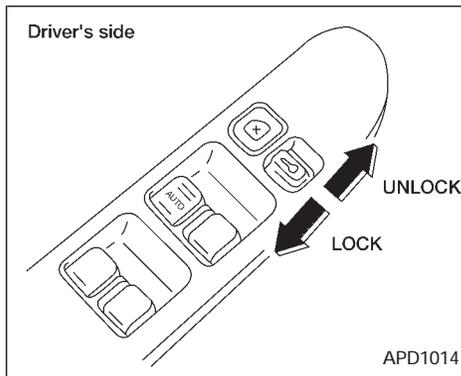
To lock from the outside without a key, push the door lock button (driver side only) or the door lock knob (driver or front passenger side), then close the door. When locking the door this way, be certain not to leave the key inside the vehicle. If the key is left in the ignition, all doors will unlock automatically.
