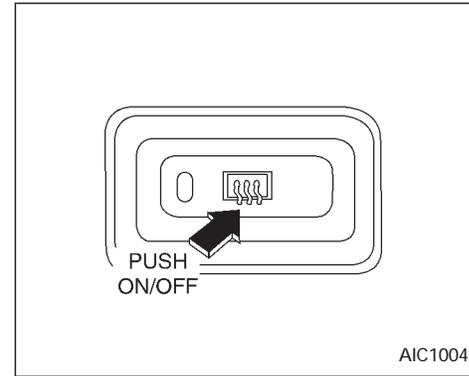
To defog the rear window glass, start the engine and push the rear window defogger switch on. The rear window defogger indicator light on the switch comes on. Push the switch again to turn the defogger off.
