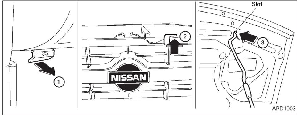
1. Pull the hood lock release handle ① located below the driver side instrument panel; the hood springs up slightly.
