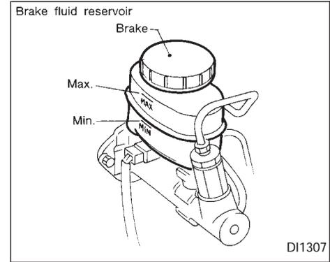
Check the brake fluid level in the reservoir. If the fluid level is below the MIN line or the brake warning light comes on, add **DOT 3** fluid up to the MAX line. If fluid must be added frequently, the system should be thoroughly checked by an authorized NISSAN dealer.
